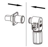
Note: Press the position indicated in the figure above before disconnecting the power terminal.
