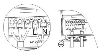
**Note:** The grounding wire shall be as thick as possible (cross-sectional area is not less than4mm²). The grounding point shall be as close as possible to the all-in-one solar charge inverter. The shorter the grounding wire, the better.
